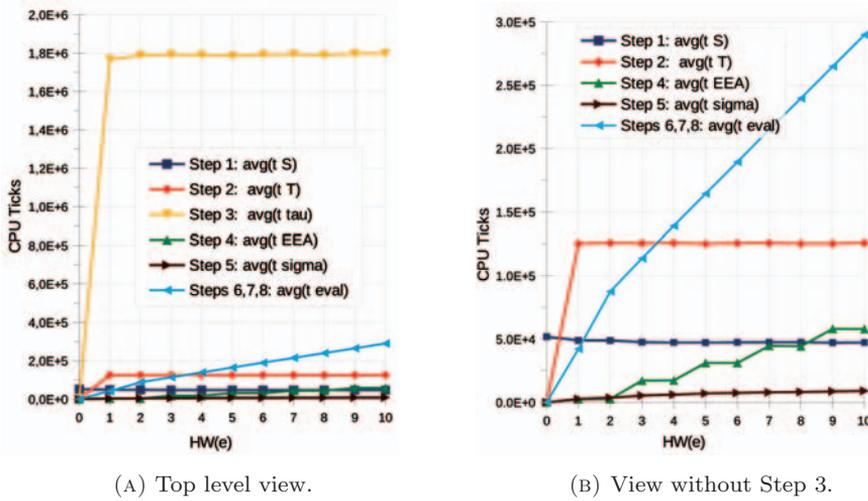
FIGURE 4. Computation time of Patterson's algebraic decoding algorithm with respect to  $w_H(e)$ . Measurements are averages based on 10 random instances of Goppa MECS with reduced parameters ( $m = 8$ ,  $n = 256$ ,  $t = 10$ ).
